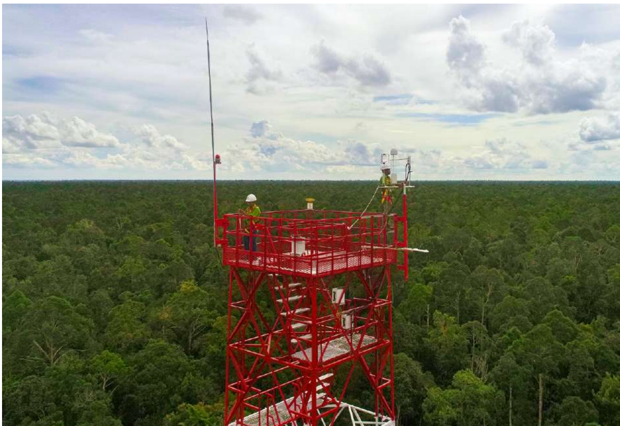
→ Greenhouse gas (GHG) tower positioned in RER to measure GHG emissions flux from the surrounding environment
